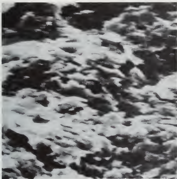
FAST CRACK PROPAGATION (5000X)
